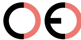
False CE Mark (too far)
